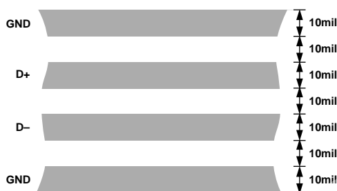
Figure 14. Arrangement of Signal Tracks
