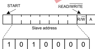
Figure 3-6. Control byte allocation
