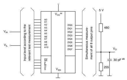
ab: In measurement of  $\rm t_{\rm dis}\textsc{-}times$  and  $\rm t_{\rm en}\textsc{-}times$  the capacitance is 5 pF.
