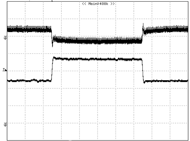
Figure 9: Output voltage response to step-change in load current (50%-75%-50% of I_{o,max} ; di/dt = 1A/\mu s ). Load cap: 10\mu F tantalum capacitor and 1\mu F ceramic capacitor. Top Trace: V_{out} (200mV/div, 200us/div), Bottom Trace: I_{out} (10A/div). Scope measurement should be made using a BNC cable (length shorter than 20 inches). Position the load between 51 mm to 76 mm (2 inches to 3 inches) from the module.
