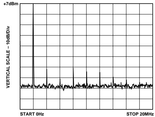
Figure 48. THD of Low Distortion Line Driver at 2 MHz
