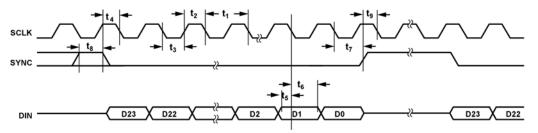
Figure 1. Timing Diagram
