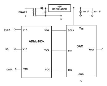
Figure 31. AD5062/AD5063 with An Opto-Isolated Interface
