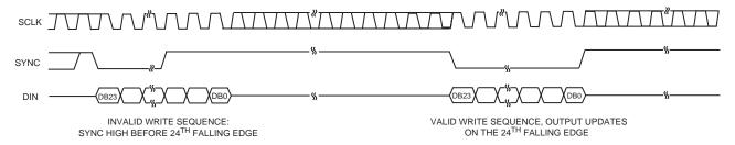
Figure 23. SYNC Interrupt Facility
