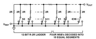
Figure X. DAC Ladder Structure
