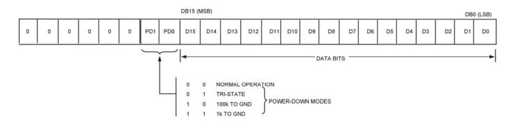
Figure 22. Input Register Contents
