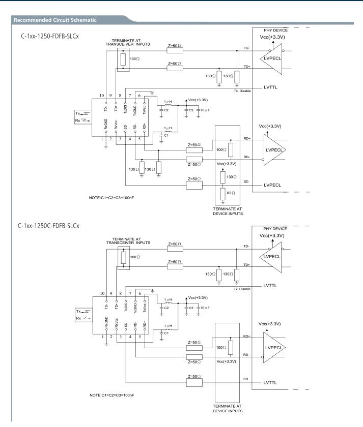
The split-loaded terminations for ECL signals need to be located at the input of devices receiving those ECL signals. The power supply filtering is required for good EMI performance. Use short tracks from the inductor L1/L2 to the module Rx Vcc and Tx Vcc. A GND plane under the module is required for good EMI and sensitivity performance.
