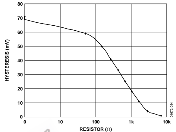
Figure 29. Comparator Hysteresis vs. R_{HYS} Control Resistor
