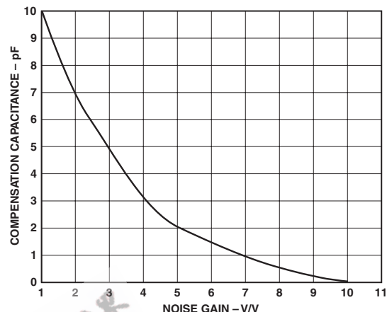
Figure 4. Suggested Compensation Capacitance vs. Gain for Maintaining 1 dB Peaking
