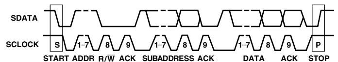
Figure 52. Bus Data Transfer
