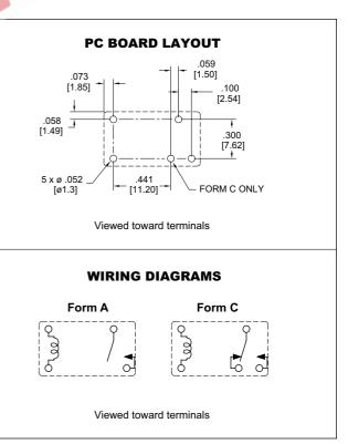
Dimensions in inches with metric equivalents in parentheses. Tolerance:  $\pm .010$ "
