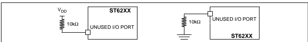
Figure 62. Two typical Applications with unused I/O Pin
