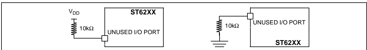
Figure 62. Two typical Applications with unused I/O Pin
