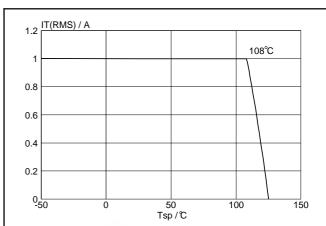
Fig.4. Maximum permissible rms current  $I_{\text{T(RMS)}}$ , versus solder point temperature  $T_{\text{sp}}$ .
