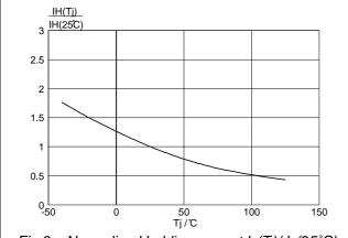
Fig.9. Normalised holding current  $I_H(T_i)/I_H(25^{\circ}\text{C})$ , versus junction temperature  $T_j$ .
