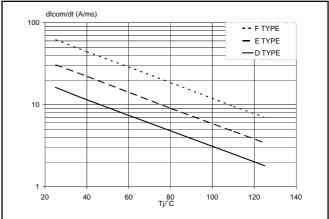
Fig.12. Minimum, critical rate of change of commutating current  $dI_{com}/dt$  versus junction temperature,  $dV_{com}/dt = 20V/\mu s$ .
