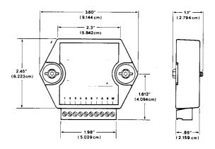
**NOTE**: Spacing for mounting screws = 2.700" (6.858 cm). Screw threads are 6 X 32.
