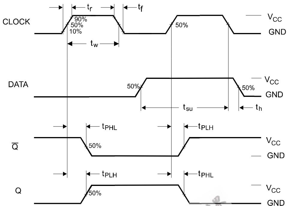
Figure 1. Switching Waveforms
