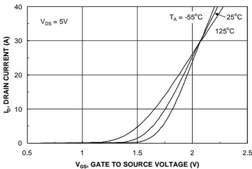
Figure 5. Transfer Characteristics.
