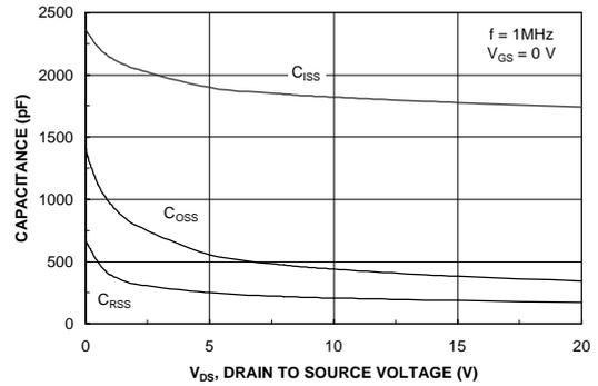
Figure 8. Capacitance Characteristics.
