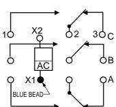
**NOTE:** Polarity must be observed with DC coil supply. Relay is polarized with a permanent magnet and will not operate or be damaged by reverse polarity.
