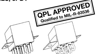
The Series FCA-325 relay is a polarized single-side stable design, where the flux from a permanent magnet provides the armature holding force in the deactivated state, and its flux path is switched and combined with the coil flux in the operated state. This results in appreciably increased contact pressure in both states over that of a spring return nonpolar design. We also manufacture other versions of this relay:
