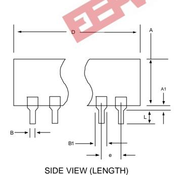
**Package Dimensions for** 40 Lead PDIP (600 mil.)
