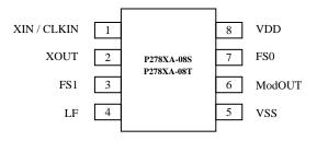
Standard pin Configuration offered in both 8 pin SOIC and TSSOP Packages
