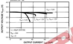
**OUTPUT VOLTAGE vs. OUTPUT CURRENT**
