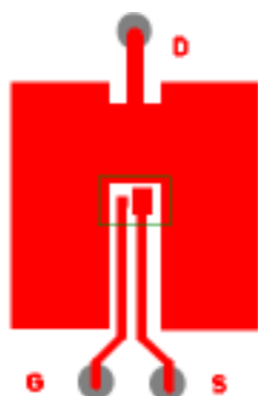
③ Surface mounted on 1 in. square Cu (still air).
