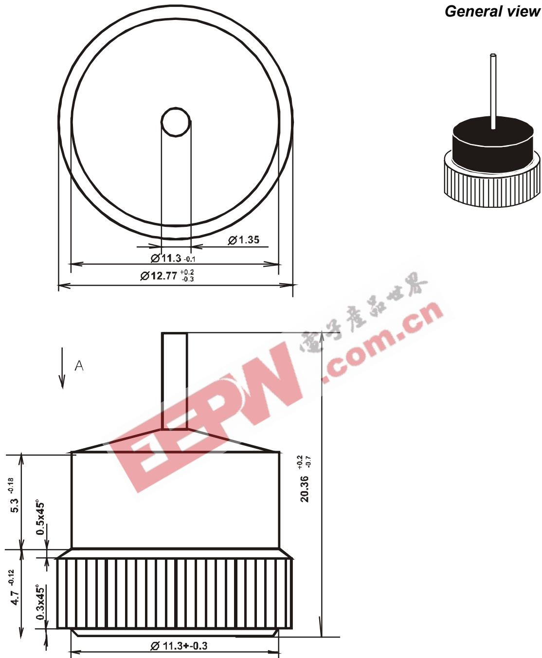
All linear dimension are in millimeters
