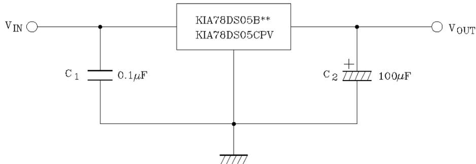
Capacitor C2 must be guaranteed to operate of the temperature range that the regulator should be operated correctly, 100 $\mu F$  is a suitable value to suppress the oscillation phenomenon at the output terminal.
