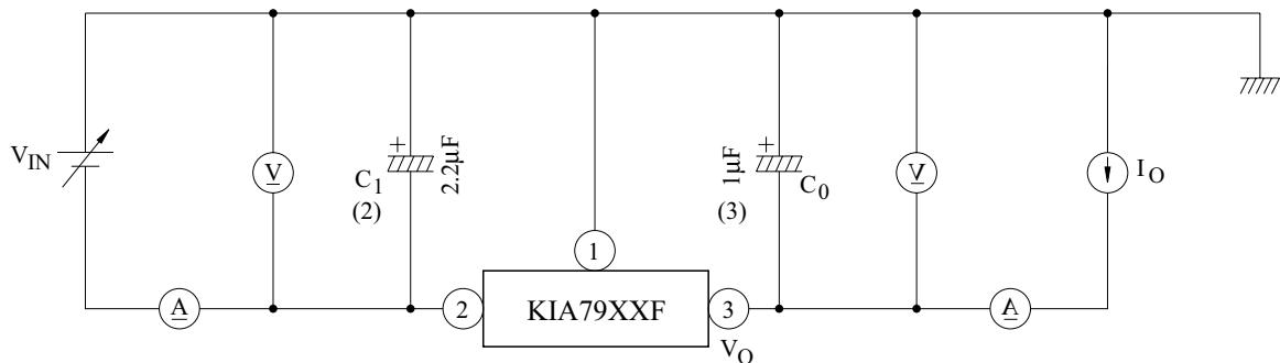
Notes : (1) To specify an output voltage, substitute voltage value for "XX"
