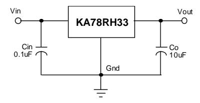
An input capacitor, Cin is not necessary for stability, but it will improve the overall performance
