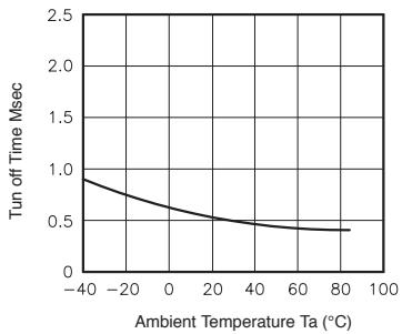
**Fig.5** LED operate vs. ambient temperature
