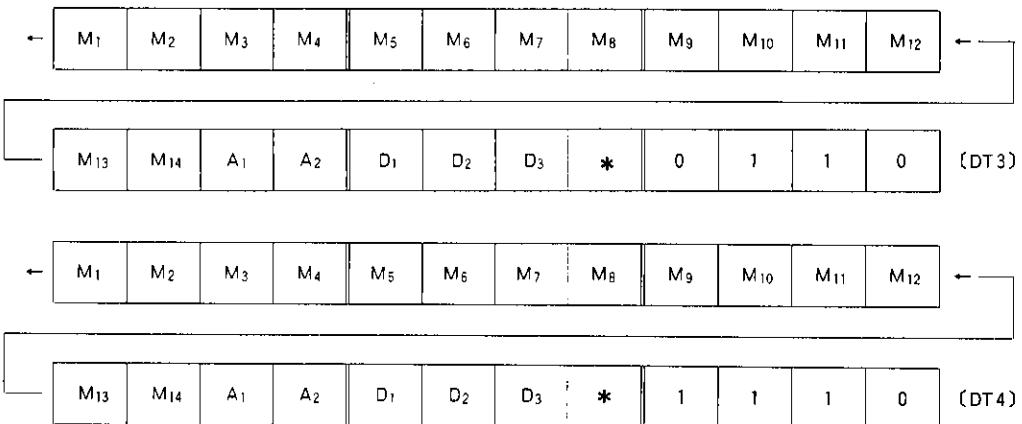
M<sub>1</sub> to M<sub>14</sub> :Display data directly used to drive segments to generate any segment pattern. These bits are not input to the PLA character generator.
