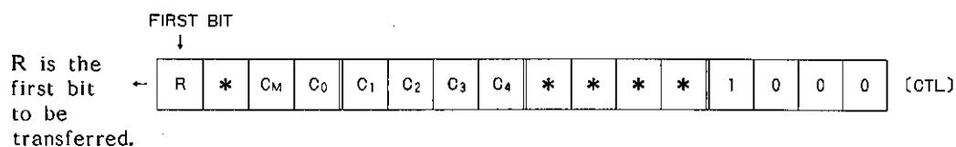
R : Resets the LSI. This serial data places the AD converter and the LCD drivers in halt mode operation.
