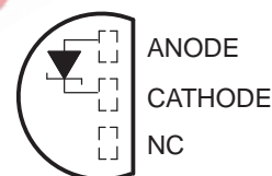
LP (TO-92/TO-226) PACKAGE (TOP VIEW)
