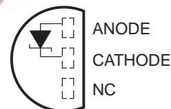
LP (TO-92/TO-226) PACKAGE (TOP VIEW)
