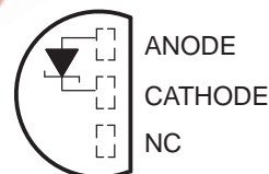
LP (TO-92/TO-226) PACKAGE (TOP VIEW)
