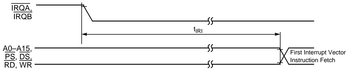
Figure 10-8 Interrupt from Wait State Timing
