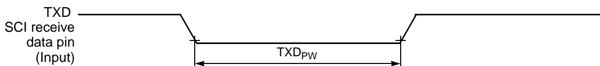
Figure 10-17 TXD Pulse Width
