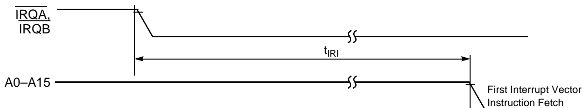
Figure 10-7 Interrupt from Wait State Timing
