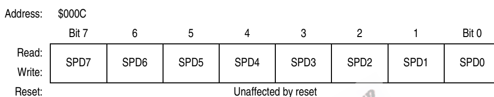
Figure 10-6. SPI Data Register (SPDR)
