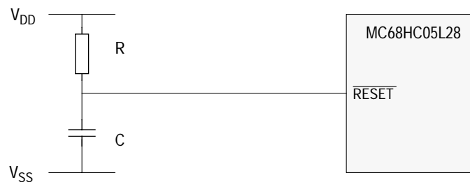
Figure 2-4 RC connection for external POR
