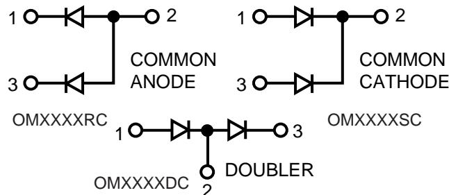
Common cathode is standard. Contact the factory for performance characteristics for common anode and doubler.
