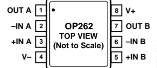
Figure 4. 8-Lead TSSOP (RU Suffix)
