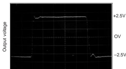
Output Voltage - 5Vp-p, 5ns/DIV
