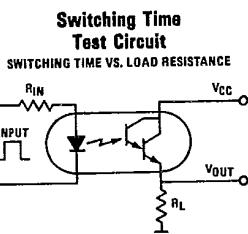
NOTE: Rise Time ( $t_r$ ) is time required for collector current to increase from 10% to 90% of its final value. Fall Time ( $t_f$ ) is time required for the collector current to decrease from 90% to 10% of its initial value.
