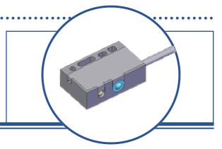
The OPB720 is a reflective switch designed to detect objects as far away as 24" (610 mm). Detectable object sizes can be as small as 0.08" (2mm) at a distance of 8" (20 mm). The OPB720 has a logical output that switches from a high level with no reflection target to a low level with a reflection target. With the addition of hysteresis, the OPB720 minimizes switching oscillations on the output. The open collector output transistor and power requirements is compatible with most PLC's
