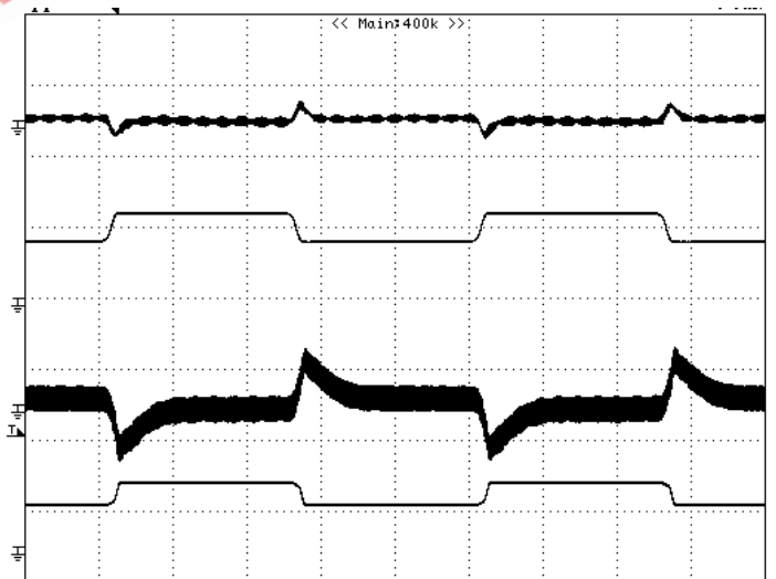
Figure 12: Output voltage response to step-change in load current I_{out2} and I_{out1} (75%-50%-75% of I_o , max; di/dt = 0.1A/\mu s ). Load cap: 10\mu F , tantalum capacitor and 1\mu F ceramic capacitor. Ch1= V_{out1} (100mV/div), Ch2= I_{out1} (5A/div), Ch3= V_{out2} (100mV/div), Ch4= I_{out2} (5A/div). Scope measurement should be made using a BNC cable (length shorter than 20 inches). Position the load between 51 mm to 76 mm (2 inches to 3 inches) from the module.
