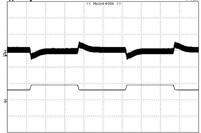
Figure 10: Output voltage response to step-change in load current I_{out2} (75%-50%-75% of I_o , max; di/dt = 0.1A/\mu s ) at I_{out1}=0A . Load cap: 10\mu F , tantalum capacitor and 1\mu F ceramic capacitor. Ch1= V_{out2} (100mV/div), Ch2= I_{out2} (5A/div). Scope measurement should be made using a BNC cable (length shorter than 20 inches). Position the load between 51 mm to 76 mm (2 inches to 3 inches) from the module.
