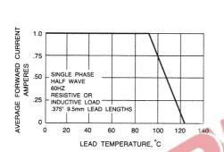
Fig. 1 - FORWARD CURRENT DERATING CURVE
