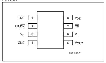
Increment ( $\overline{INC}$ ) is an edge triggered input. Whenever  $\overline{CS}$  is low and a high to low transition occurs on the  $\overline{INC}$  input, the  $V_{OUT}$  voltage will either move toward  $V_H$  or  $V_L$  depending upon the state of the  $UP/\overline{DN}$  input.
