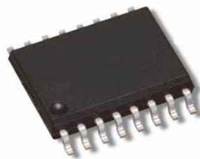
Figure 1 : Image of TSSOP -16 Exposed Paddle Plastic Package
