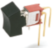
T101J1AVBE2 Vertical Actuation SPDT
