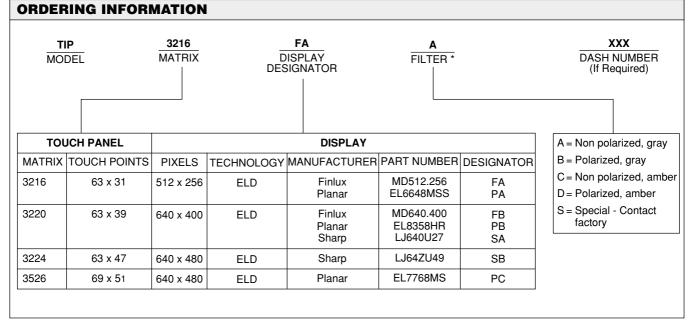
\*Other user specified filters will be designated as "S". Contact factory for availability. Any "S" filter designation will require a factory assigned dash number suffix. Filters A-D are plastic. Glass filters may be available on selected models. **Note:** Many additional touch panel options available to fit color LCD's and other display technologies. Please contact factory for assistance.
