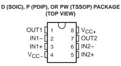
The TL3414A device is a dual operational amplifier that can be operated with single or dual power supplies. In addition to high gain and high output voltage swing, it is capable of driving a 70-mA load, making it ideally suited for simple, low-cost audio-amplifier applications, such as headphone amplifiers in DVD and CDRW applications.
