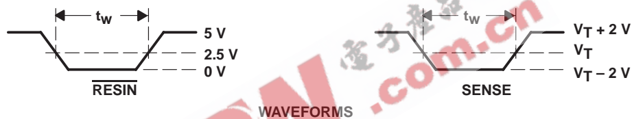
Figure 2. Input Pulse Definition
