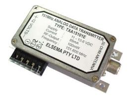
The TXA15101E is an analog and digital 151 MHz transmitter. The analog signal, normally 4-20mA is transmitted and then recreated at the receivers (RXA15101E) analog output. Also, the normally open digital contact can be simultaneously transmitted with the analog signal. This eliminates the high cost of wiring and has the flexibility of wireless data collection.
